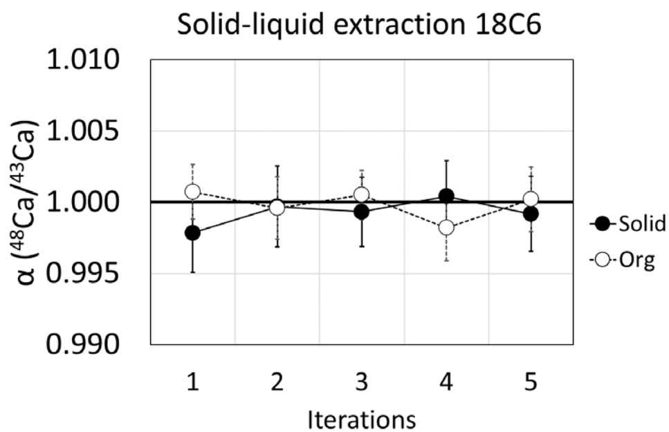
Fig 3.36 The separation factor ( \alpha ) of solid-liquid extraction and a multistage iteration using 18C6.
