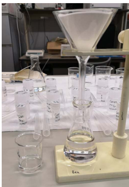
Fig 2.4 Phase separation using filter
