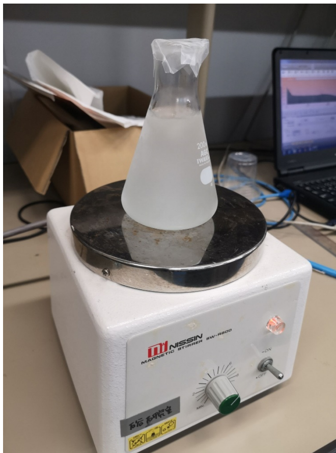
Fig 2.2 The mixing of organic and aqueous phase by magnetic stirrer
