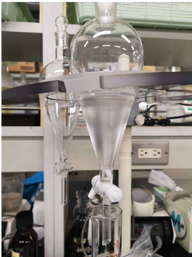
Fig 2.3 Phase separation in separation funnel
