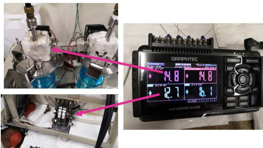
Fig 3.47 The temperature logging system on the Peltier and the electric plates.
