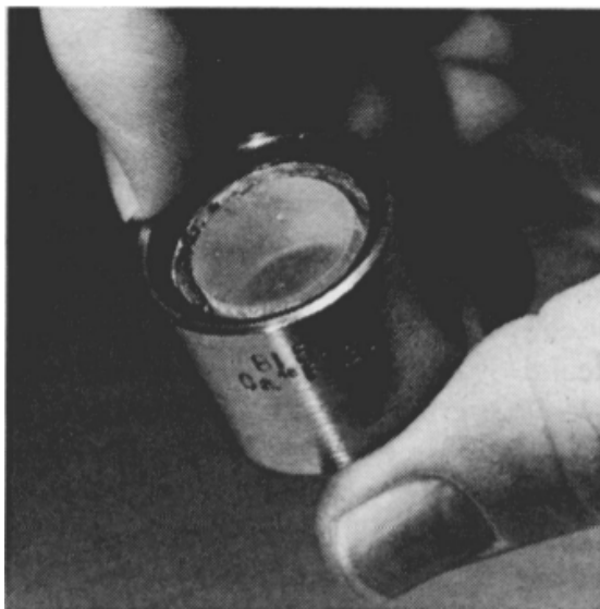
Fig 1.18 ^{48}\text{CaF}_2 crystal produced by Calutron for the study of double beta decay [56]
