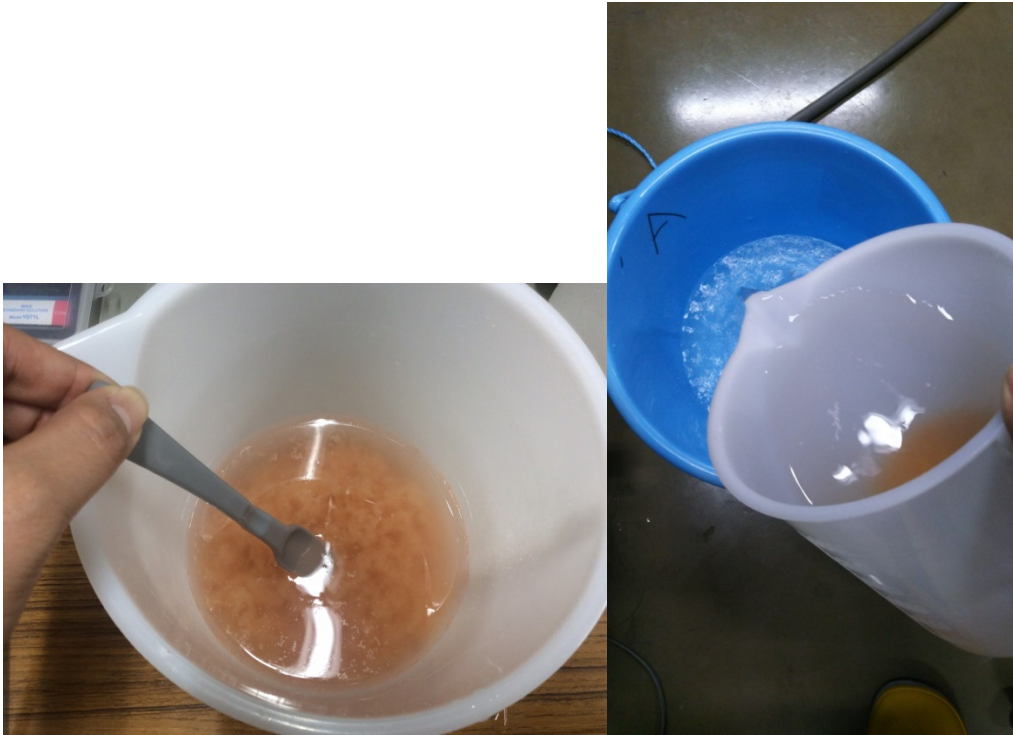
Fig 2.28 Mix the resin in pure water and pour the water out of the resin.
