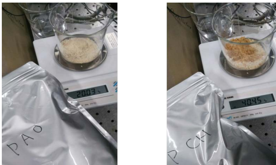
Fig. 2.25 PAO resin ( \text{OH}^- form): Powdered hydroxide form anion exchange resin PCH resin ( \text{H}^+ form)): Powdered hydrogen form cation exchange resin.
