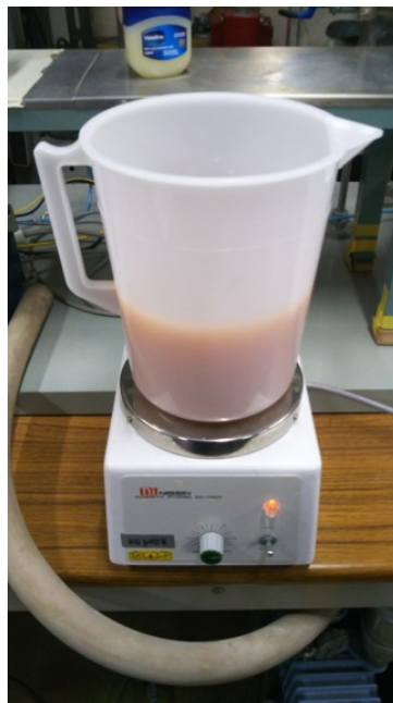
Fig 2.29 Mix the resin with 30 minutes stirrer.
