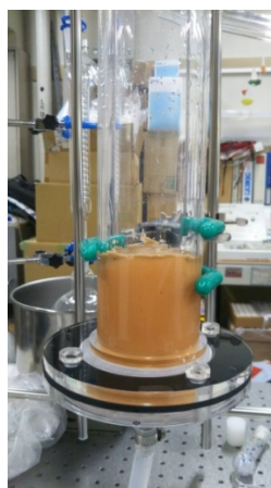
Fig. 2.33 Wait for 20 minutes after all sample pass through the resin.
