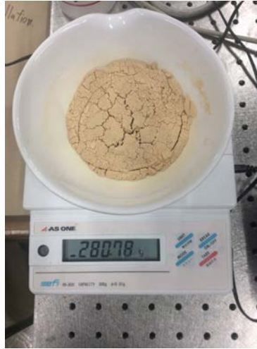
Fig. 2.34 The dried homogenous resin that contain ^7\text{Be} and ^{210}\text{Pb} .
