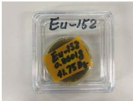
Fig. 3.12 The standard source Eu-152 0.8601 g , 20mm diameter and around 2mm thickness activity is 41.75 Bq.
