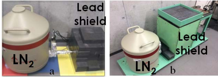
Fig. 2.3 The HPGe detector with liquid nitrogen and (a) the period lead shield system and (b) new lead shield system.
