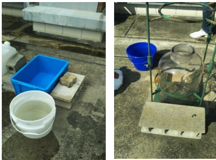
Fig. 2.24 A small basin with an open with an open surface area of 0.14 \text{ m}^2 (left side) for total deposition dust fall sample the collection area of 0.07 \text{ m}^2 for wet deposition (right side).
