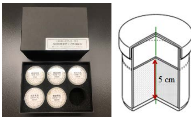
Fig. 2.10 The standard source is MX033U8PP set, the cross section of standard source No. 4132-5cm.
