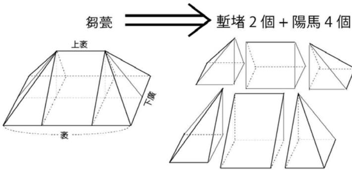
$$2 \times \text{下表} \times \text{下廣} \times \text{高} = \text{堑堵} 8 \text{ 個} + \text{陽馬} 24 \text{ 個}$$
