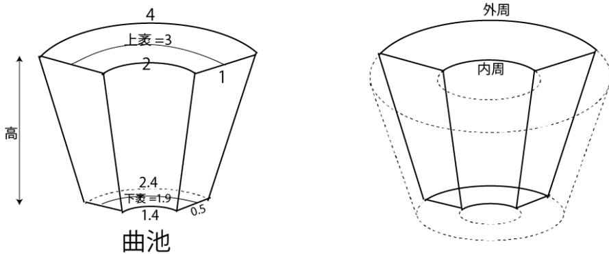
$$\text{体積} = \{(2\text{上表} + \text{下表}) \times \text{上広} + (\text{上表} + 2\text{下表}) \times \text{下広}\} \times \text{高} \div 6$$
