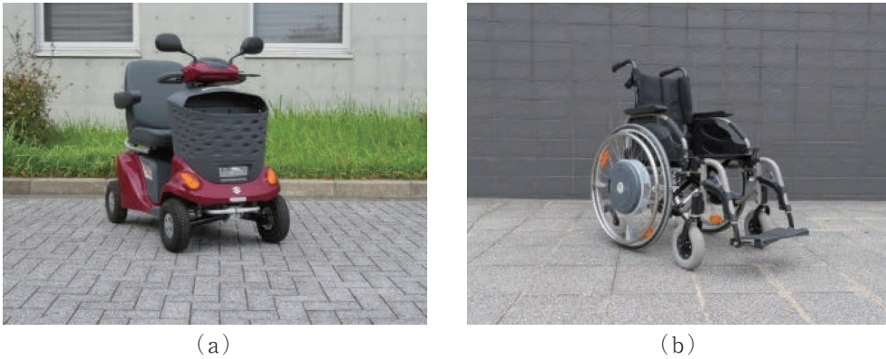
Fig. 2 In the experiment, we use a handle type electric wheelchair, and a power assist wheelchair. (a) is a Suzuki handle type electric wheelchair "ET 4 D" made by Suzuki. (b) is an power assist wheelchair "e-motion" made by ALBER.
