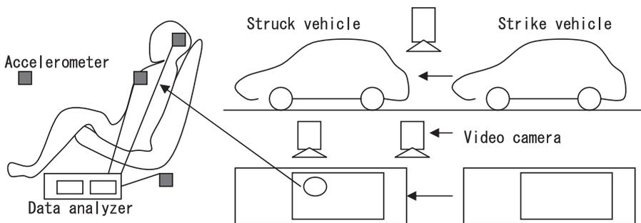
Fig.4 Schematic diagram of collision experiment
