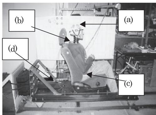
Fig.9 Sled view and the part equipped with the accelerometer
