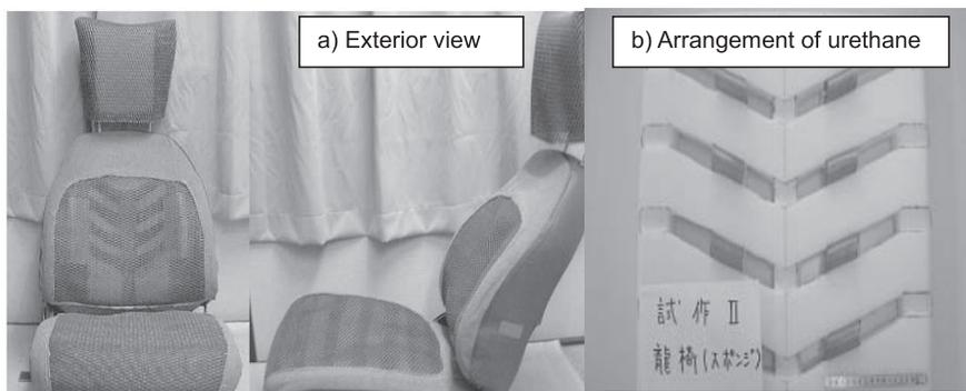
Fig.15 View of the back of the proposal seat
