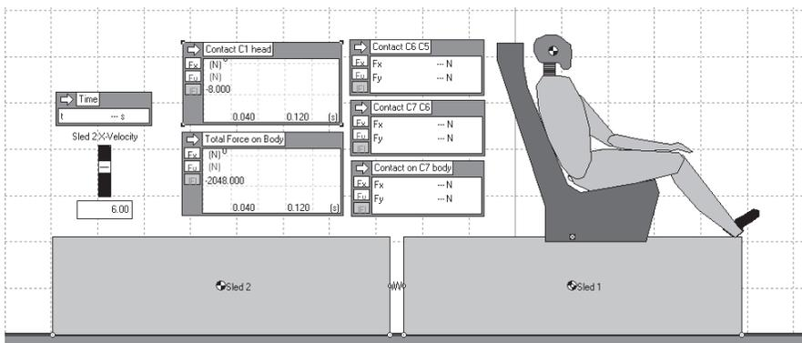
Fig.13 A model which simulates the simple actual vehicle collision
