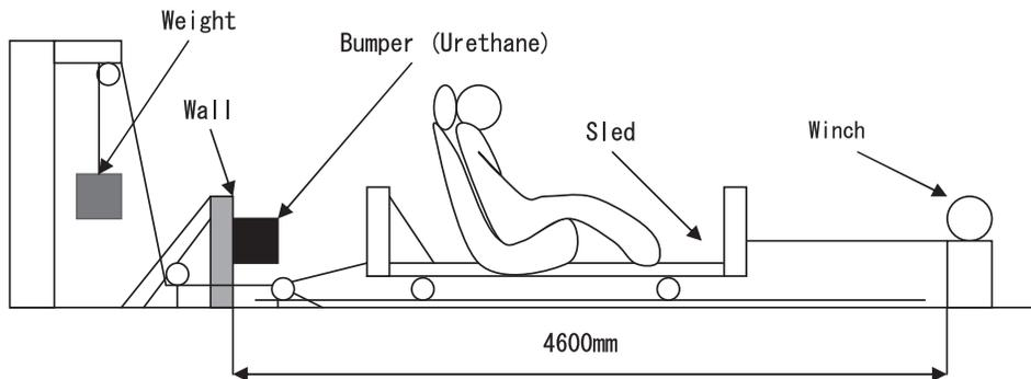
Fig.8 Schematic diagram of the sled type collision apparatus
