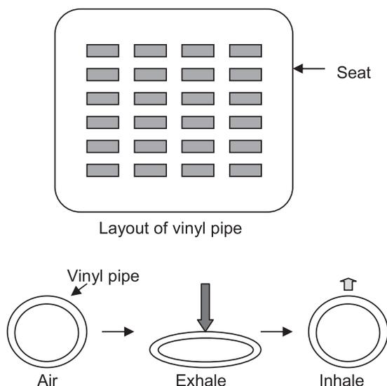
Fig.18 Pumping mechanism to self-breathing
