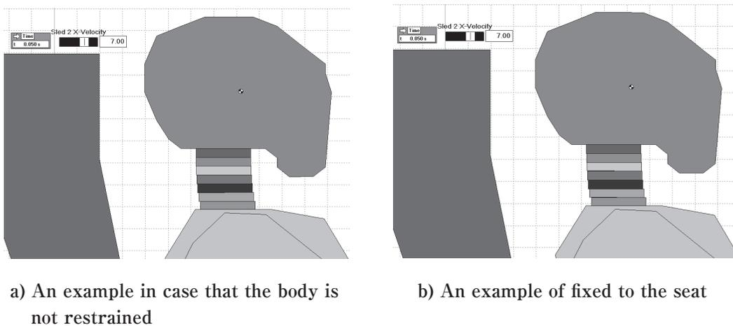
Fig.14 Deformation patterns of the neck
