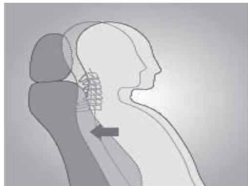
Fig.3 A type of seat that catches shoulder parts softly
